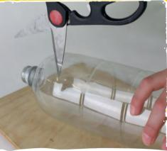
Then to enlarge the hole, use a sharp, pointed pair of scissors. Place one end of the scissors into the small hole you have made and, being careful, use a twisting action to open up the hole to the right size.
